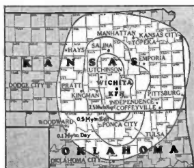
Glenn D. Gillet's Computed Field Strength Distribution Based on Performance and Previous Survey Measurements—5000 Watts Day and Night—October 1941
